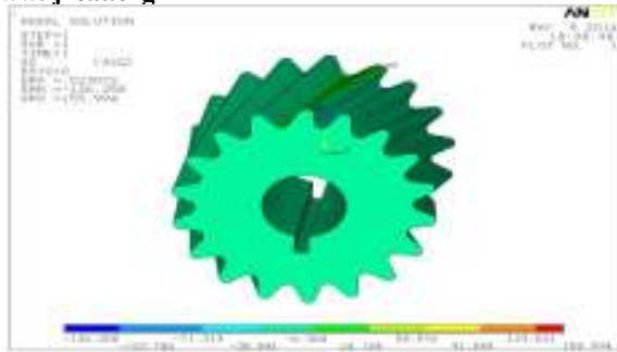
Fig 7.10: Bending stress of Helical Gear with ceramic as material
