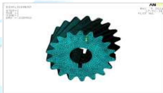
Fig: Deflection of Helical Gear with ceramic as material
